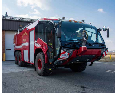
Station 33's new 38.5 ton Rosenbauer Panther P-23 crash truck is parked outside of its bay on 4-March-2021. The new truck greatly expands the capability of the fire station to respond to air-field emergencies. It is maintained by the 166th LRS vehicle maintenance unit. (U.S. Air National Guard photo by A1C Brandan Hollis)
