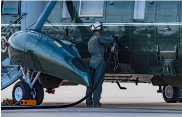
Airmen refuel Marine One on 12-March-2021. One of many missions for the 166th fuel shop, supporting POTUS aircraft presents unique logistical challenges. The unit provides fuel for the 166th Airlift Wing's own fleet of eight C-130H2 tactical airlift planes as well as Delaware National Guard Army Aviation. (U.S. Air National Guard photo by Mr. Mitch Topal)
